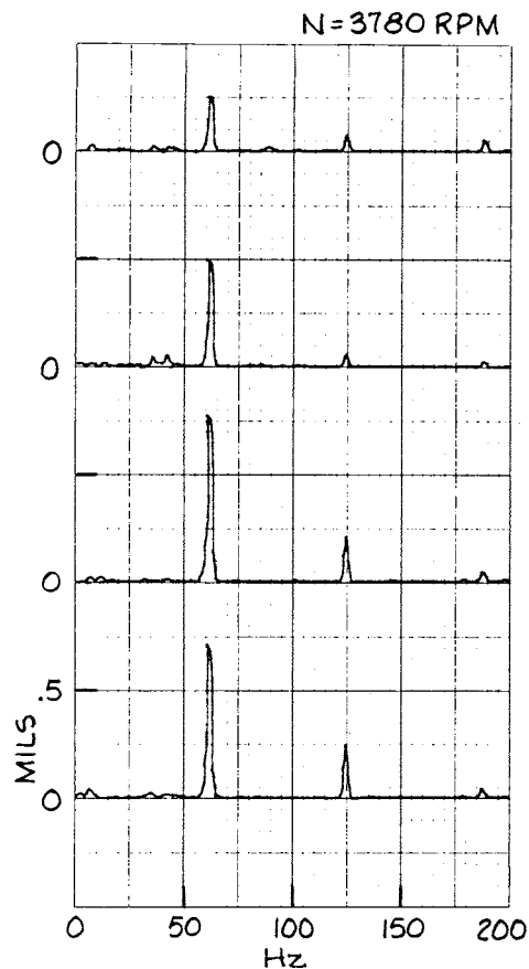
Fig. 21 Axial compressor frequency spectrum, 4 pad tilting pad bearings, N = 3780 rpm
