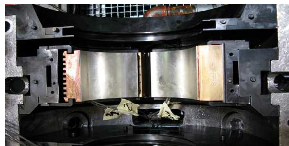
Figure 17. Ultra High Speed Application—Evacuated TPJ Bearing.
