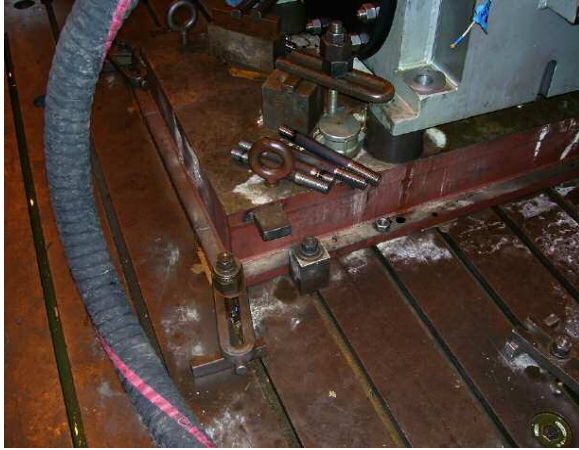
Figure 9. Original Fabricated Hollow Baseplate.
